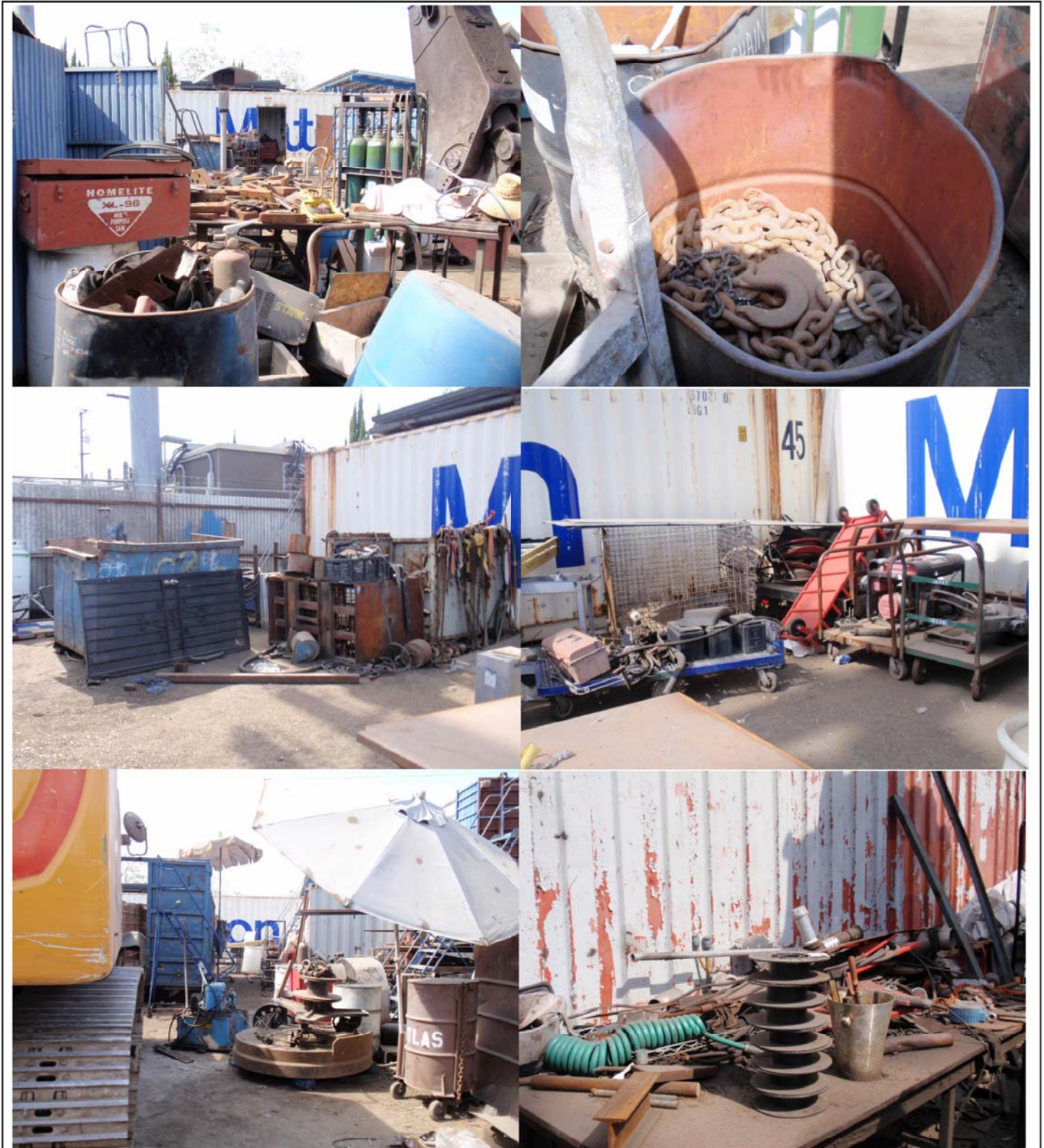
Photographs 32-37: The photographs show a maintenance area with poor housekeeping practices. This area has rusty equipment, car batteries, and debris exposed to precipitation without BMPs in place.
