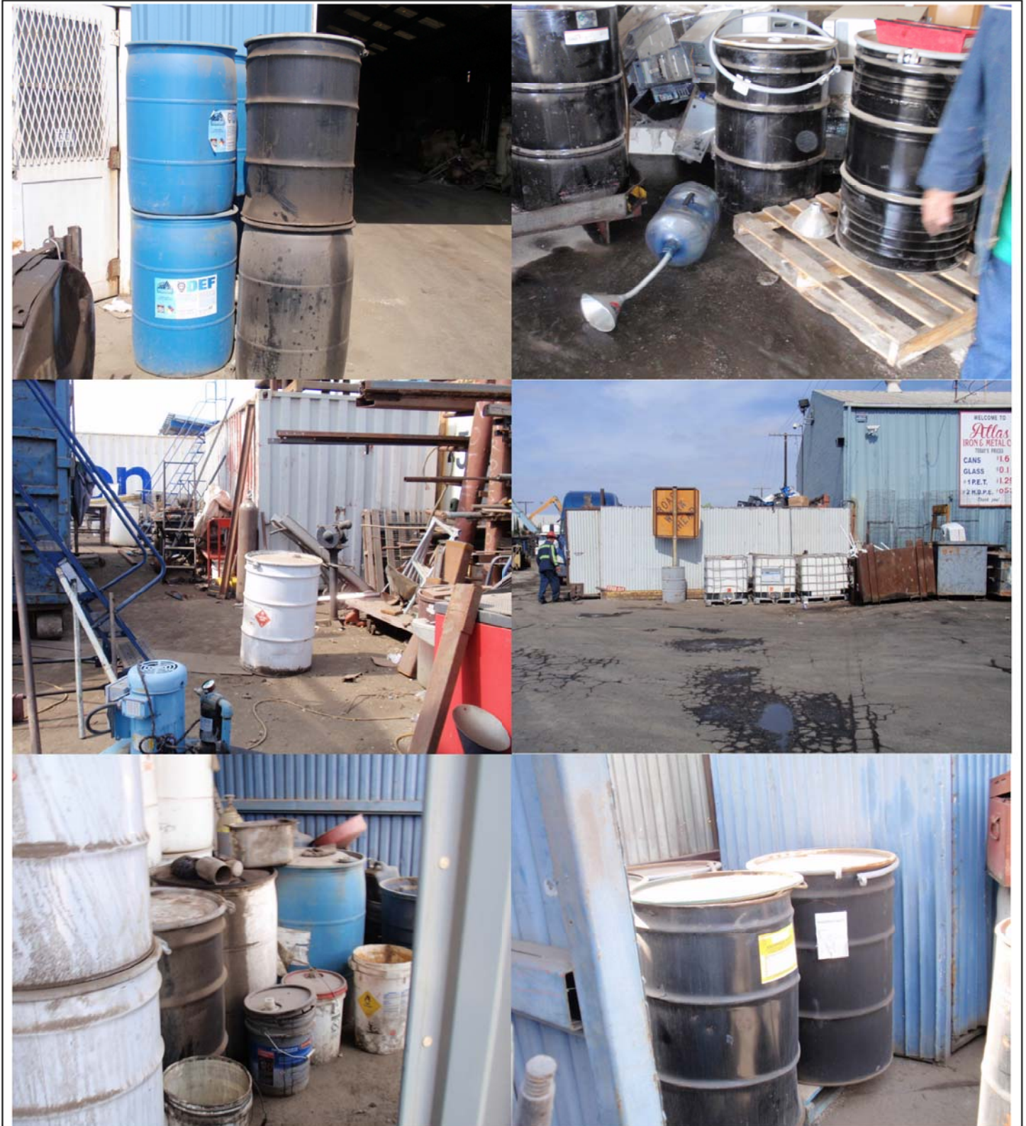
Photographs 26-31: The photographs show empty plastic drums, metal drums, tote tanks, and other containers containing wastes without overhead cover and secondary containment.
